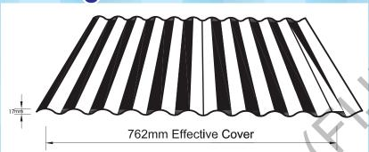
RPFL CorruDek® is the famous Australian corrugated profile. CorruDek® is equally at home with traditional and contemporary designs. It is available in three basic metal thicknesses, and is fixed with ease and speed. Use CorruDek® 0.55mm for curving famous corrugated profiles.
